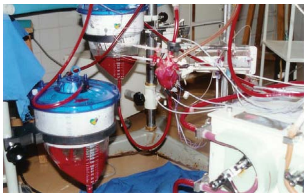
Fig.2 – Overview of the perfused isolated heart. Isolated heart with metallic mini forceps for induction of regional ischemia. LA reservoir working as preload reservoir. Venous reservoir from which the blood was reinfused toward the animal support. Afferent line of the roller pumps from the animal support. Piezoelectric crystals wires
